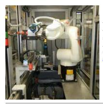
To deliver 100% CMM-like inspection for highvolume automotive component manufacturing, a supplier of V6 valve covers tapped HAHN Automation to design and build an inspection system that relies on machine vision. Read full story
